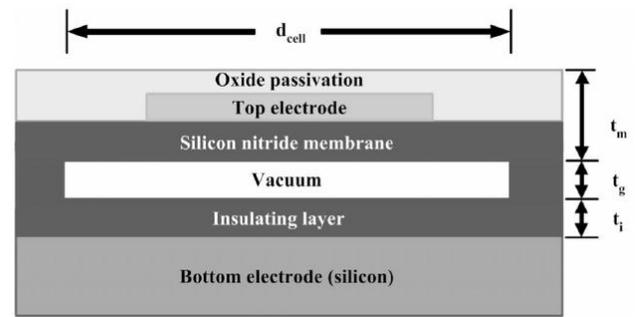
**Figure 2 Diagram of a CMUT (from Oralkan *et al.*) (6)**
