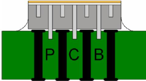
**Figure 1 Diagram of the through hole electrical connections used by Eames *et al.* (5)**
