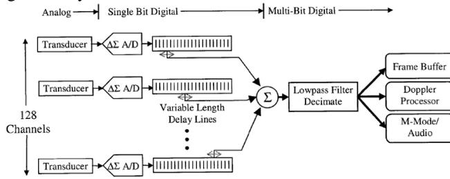
**Figure 6 Diagram of the Delta-Sigma Oversampled Beamformer (10)**
