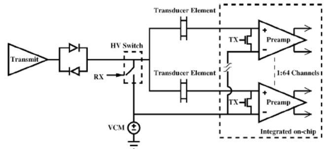
**Figure 8 Diagram of the transmit protection circuitry as described by Fuller *et al.* (14)**
