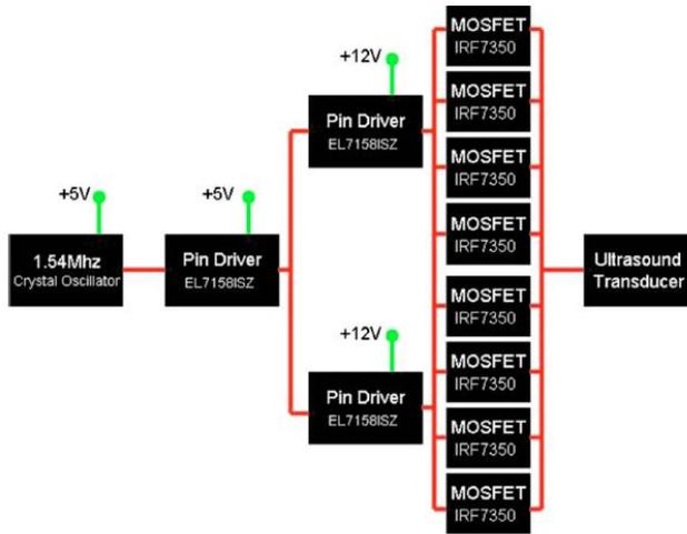
**Figure 3** Block Diagram of the circuitry used by Lewis *et al.* to provide low output impedance (8)
