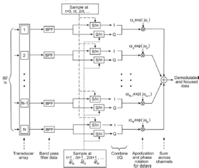
**Figure 7 Diagram of the Direct Sampled I/Q Beamforming Algorithm (13)**
