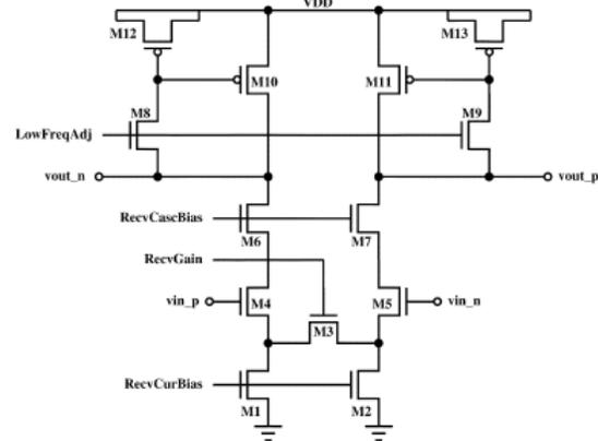
**Figure 5** Schematic of the single stage preamplifier used by Fuller *et al.* The gain can be adjusted between 30 dB and 85 dB by adjusting RecvGain (1)
