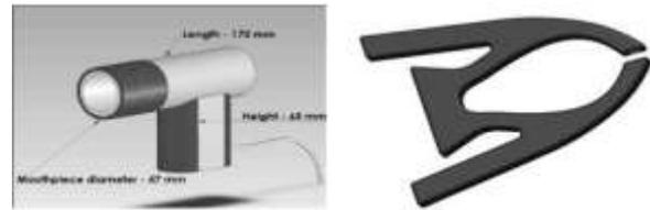
Fig. 2. Left: spirometer sensor, Right: Pulse oximeters sensor will contain light emitting diodes and a photodiode.
