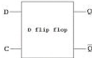
Figure 2 The symbol for a flip-flop
